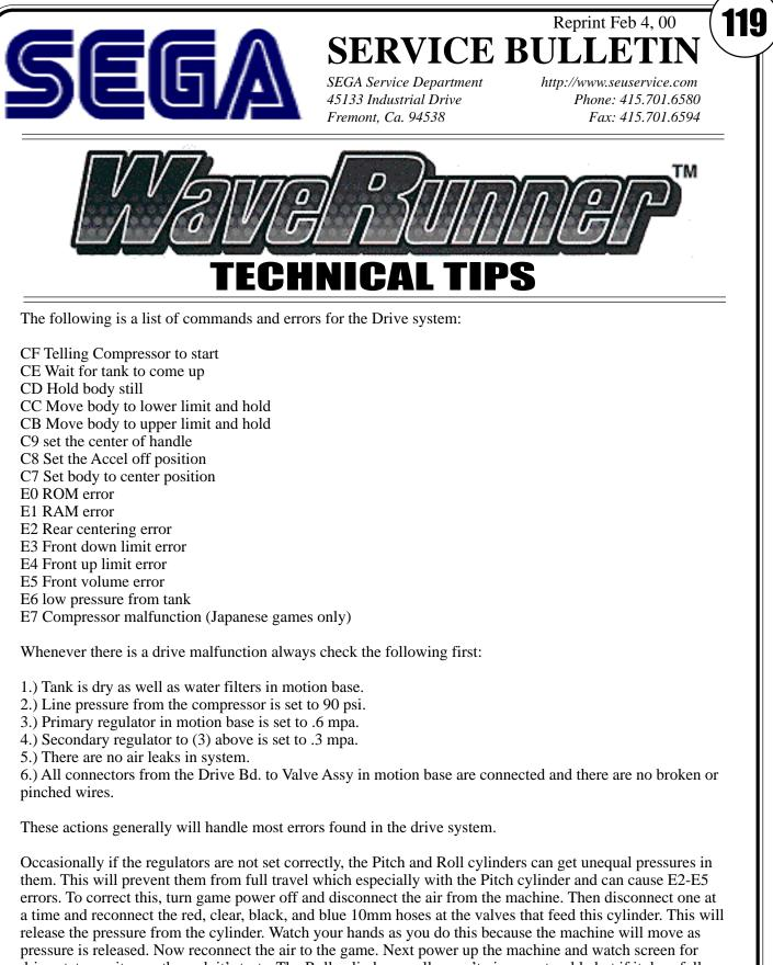
pressure is released. Now reconnect the air to the game. Next power up the machine and watch screen for drive status as it goes through it's tests. The Roll cylinder usually won't give you trouble but if it does follow the same procedure with the exception of disconnecting the four 10mm hoses. There will be one small green 6mm and one small yellow 6mm hose that goes over to the Roll cylinder. These can be disconnected at the two valves in the Roll valve area.
