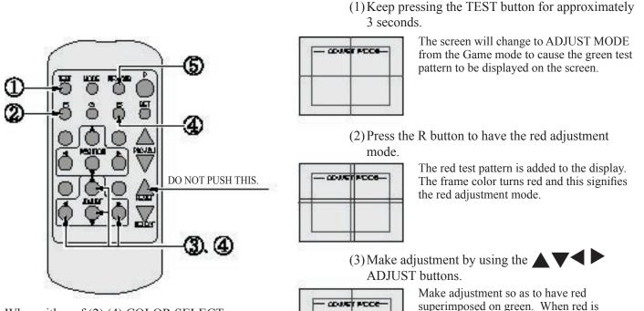
When either of (2) (4) COLOR SELECT buttons (R, B) is pressed, if the color desired to be adjusted disappears, press that particular button again. For example, if the red color needs to be adjusted again at the stage of (4), the R button need to be pressed twice.
