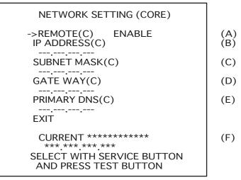
Use the SERVICE Button to move the cursor to the desired test item. (When setting IP ADDRESS, SUBNET MASK, GAME WAY or PRIMARY DNS, use the underline as a guide.)
