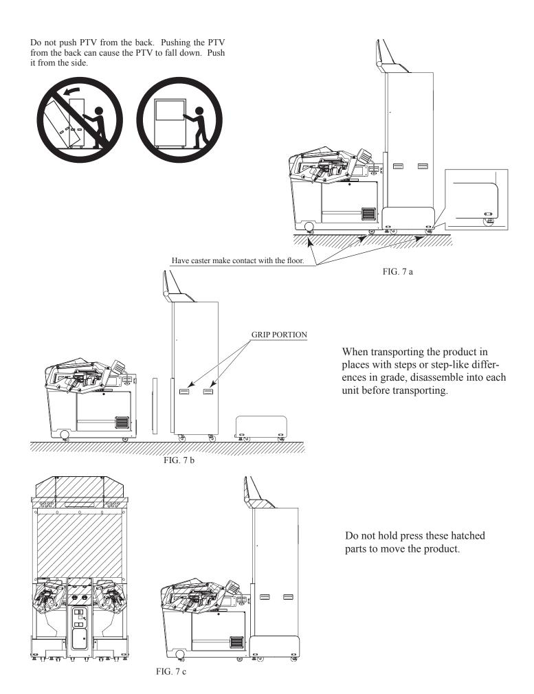
Do not tie machine down using Plastic Parts as an anchor. When using straps or tie downs (rope etc), use caution. Use protective material where tie downs contact machine to avoid damage.
