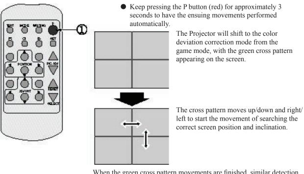
When the green cross pattern movements are finished, similar detection is performed sequentially in order of red and then blue cross movements. After detecting by green, red and blue cross movements, the game mode returns with the color deviation status being corrected.
