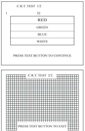
In the TEST mode menu, selecting C.R.T. TEST allows the screen (on which the projector is tested) to be displayed. Although the projector adjustments have been made at the time of shipment from the factory, make judgment as to whether an adjustment is needed by watching the test mode screen. If it is necessary, adjust the projector by referring to Section 12.
