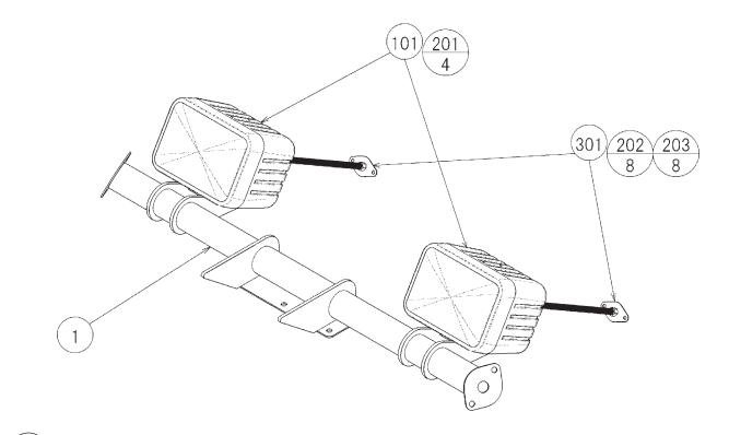
Attach (101) so that the speakers are on the outside and the bass reflex ducts are on the inside.
