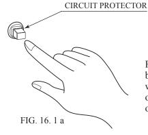
Functions due to the activation of bimetal. To restore the function, wait for approximately one minute or longer until the bimetal cools off. (Press the Button.)
