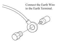
FIG. 6. 7 b \*Earth Wire Connection
