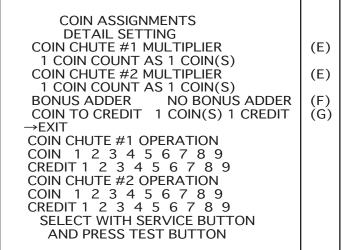
DETAIL SETTING COIN CHUTE #1 MULTIPLIER 1 COIN COUNT AS 1 COIN(S) BONUS ADDER NO BONUS ADDER COIN TO CREDIT 1 COIN(S) 1 CREDIT  $\rightarrow$ EXIT COIN CHUTE #1 OPERATION COIN 1 2 3 4 5 6 7 8 9 CREDIT 1 2 3 4 5 6 7 8 9
