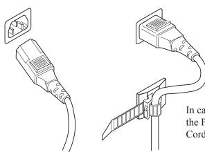
In case the Power Plug is apt to come out of place, secure the Power Cord to the periphery of the AC Unit with the Cord Clamp (an accessory).
